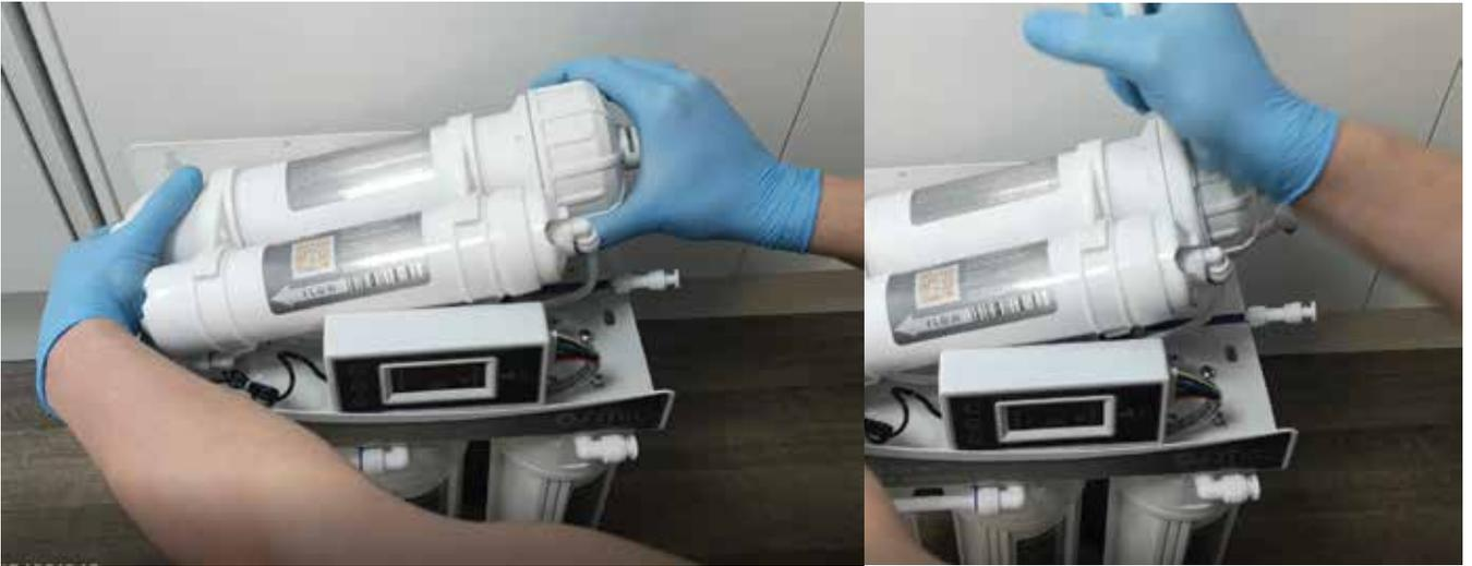
Insert the membrane into the membrane housing. Ensure it goes into the socket at the other end of the housing inside it and the membrane is flush with the top of the housing.
