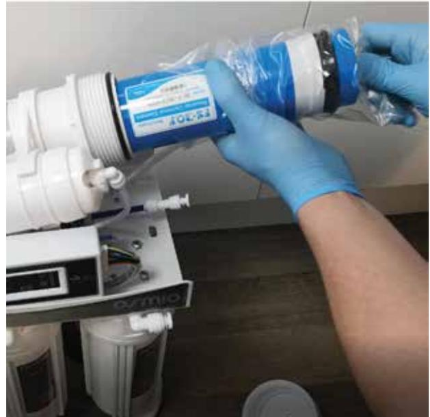
Insert the membrane into the membrane housing. Ensure it goes into the socket at the other end of the housing inside it and the membrane is flush with the top of the housing.
