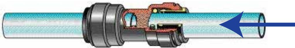
**Step 4:** Now push the tubing into the fitting harder until the tube stop is felt. The collet has stainless steel teeth which hold the tubing in position while the O-ring provides a permanent leak proof seal.
