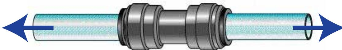
**Step 6:** To disconnect the tubing from the fitting, ensure that the system is depressurized first. Push in the collet squarely against the face of the fitting. With the collet held in this position, the tubing can be removed by pulling. The fitting and tubing can be reused.
