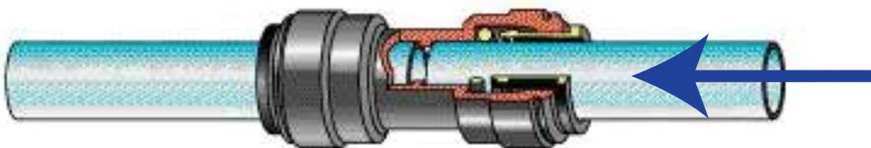
**Step 5:** Pull on the tubing away from the fitting and make sure it stays firmly in place. It is good practice to test the connection with pressurized water before finishing installation.
